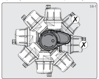
$1. The\ motor/gearbox\ is\ bolted\ via\ the\ through\ deck\ mounting\ bolts.$
