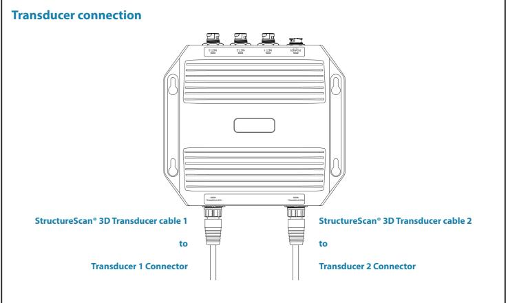
Ensure both StructureScan® 3D transducer cables
