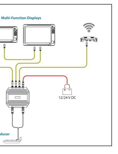
are connected to the StructureScan® 3D Module correctly
