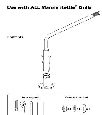
Mount may be installed on any angle horizontal surface. However, in order to use it as a rotating mount, it must be installed in a completely level position. Shims, not provided, may be used during installation to level this mount.
