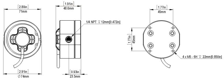
Figure 3 - Fuel Flow Sensor Mechanical Drawing
