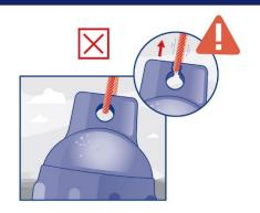
Using a line diameter that is too small can act like a knife and abrade or create friction on a single point in the ropehold causing the ropehold to crack or tear. We prefer and recommend nylon rope over other types because of its stretch properties. It is a little more forgiving and softer creating less friction. Remember, rope is much stronger than the PVC our fenders are made from, and always wins in the end.
