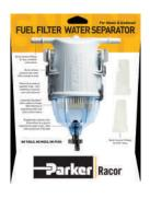
NOTE: Kits include Aquabloc media in 2, 10 or 30 micron ratings. Two micron is recommended for ultrafine filtration of solid contaminants. SNAPP fuel filter water separators are packaged for a first installation with mounting bracket and quick connect fittings. The replacement kit includes a new SNAPP filter and priming accessory.
