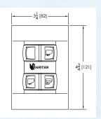
Multifunction Flush Panel Allows independant operation of intake or discharge no timed flush. Can be mounted horizontally or vertically.
