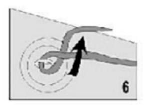
Step G. Feed the tip of the end into the center of the lifeline ropes core, while gathering the outer area to make passage easier.
