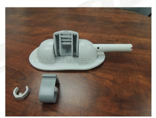
Step 6. Install the New C-Clip onto the axis.
