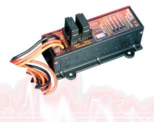
The **Battery Charger / Maintainer** enables an **extra battery bank** to be kept 'topped up' from the **main battery bank** which has the charging device(s) connected to it (e.g. alternator, battery charger, solar cell/wind turbine etc.).
