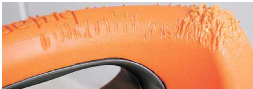
Figure 1b Abrasion damage, originating sharp edge for possible cutting of hands (level 2) – Repairable
