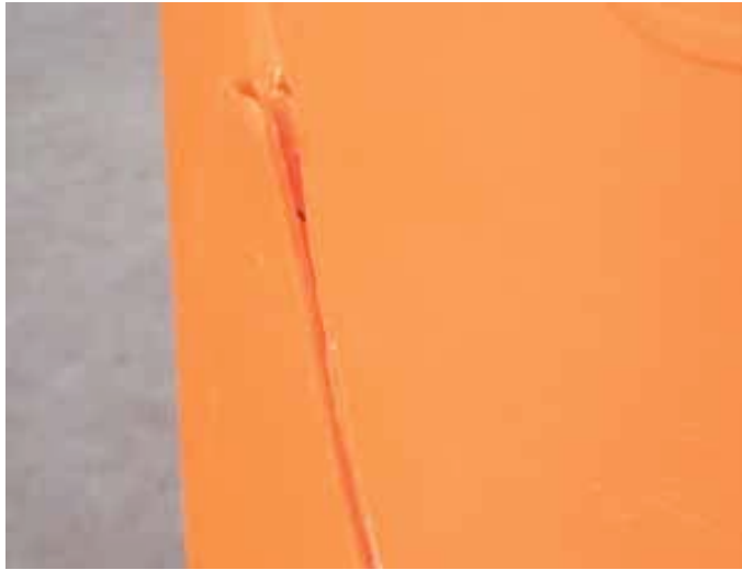
Figure 7a Cuts & Gouges (level 2) – Repairable
