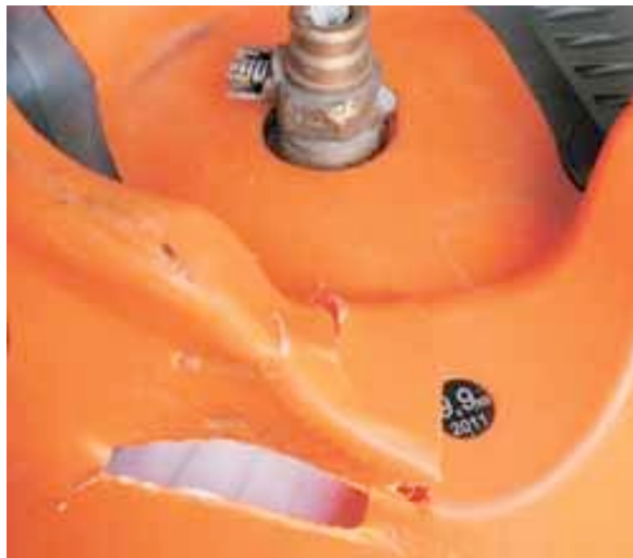
Figure 2c Impact Damage (level 3) originating valve damage distortion - Not Repairable
