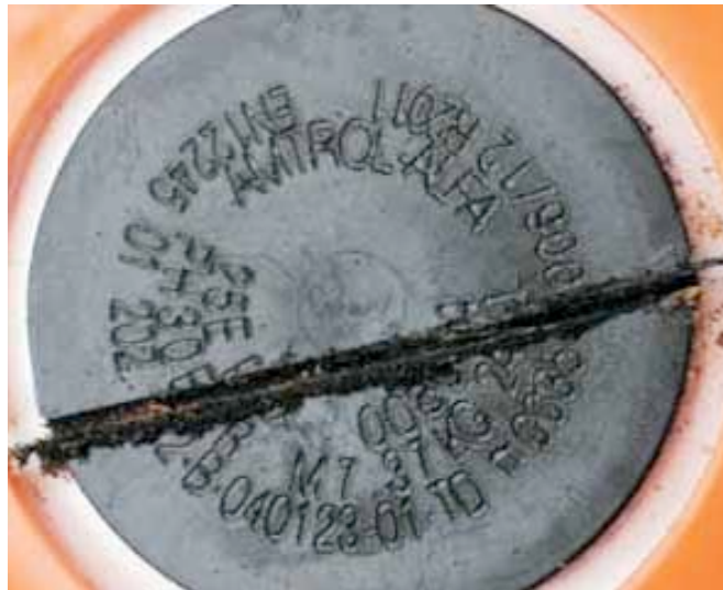
Figure 6 Marking Illegible (level 2) - Repairable
