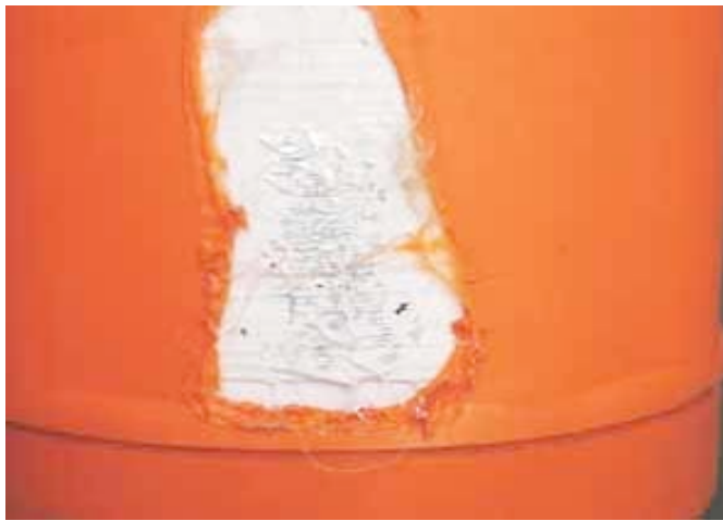
Figure 3b Heat Damage (level 3) - Not Repairable
