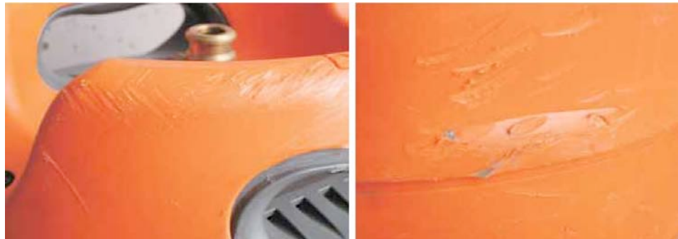
Figure 1a Abrasion Damage (level 1) – Serviceable
