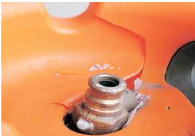
Figure 4 Structural damage (level 3) - Not Repairable
