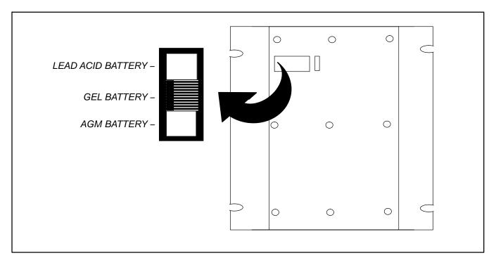
Figure 1. Battery Type Selectable Switch (Bottom View)
