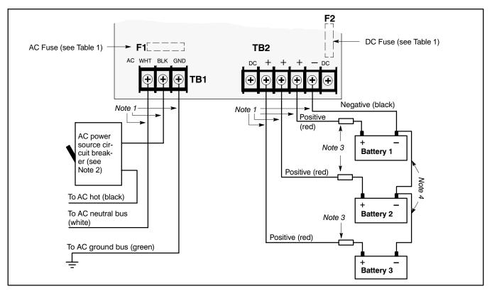
Figure 2. Wiring Diagram (Reference Table 1 for Applicable SP Series C-Charger Model)
