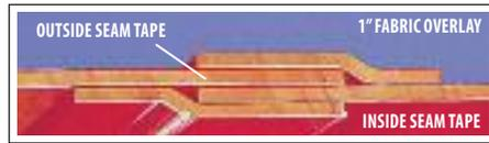
Our seams are overlapped a full inch and reinforced with seam tape both inside and out. No one else takes so many steps to ensure seams will last.
