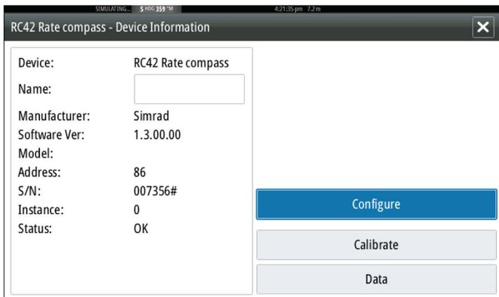
All devices allow allocation of an instance number in the configure option. Set unique instance numbers on any identical devices on the network to allow for the unit to distinguish between them. The
