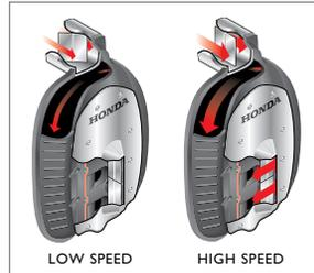
volume and velocity of air flow. It all adds up to a simple, compact design that enhances both low speed drivability and high-speed performance. **BF250, BF225, BF200, BF150, BF135.**
