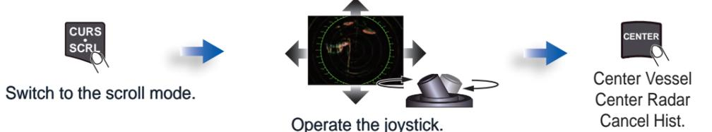
**Note:** In the cursor mode, you can pan the display by moving the cursor to the edge of the screen. This function is available in the full screen Plotter/Weather/Radar display.
