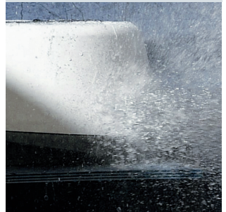
The Broadband Radar family of radomes have undergone demanding waterproof testing.
