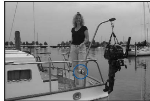
The Nova Lift™ with Winch is for boats that don't have readily available sheet winches. The height of the winch is adjustable for ease of operation.
