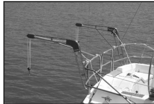
Constructed from heavy wall 304 stainless steel, and strategically sleeved to give double wall thickness in high load areas, Each davit is supplied with a cam cleat as well as a standard horn cleat for added safety.
