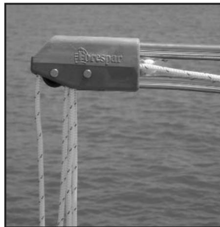
Marlon™ end heads, which incorporate quality Harken roller ball bearing sheaves, greatly add to the smooth operation and reduces the chance of the line tangling over the more common block and tackle.
