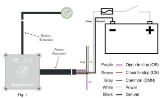
The Guardian Extension cable set can be used to extend the distance by 750mm / 29.5 inches for either the Power cable, the Switch cable or both. This is designed for use on larger vessels where the Guardian hub needs to be located further from either the control switch or the power and kill switch connections.
