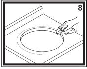
8) Clean the counter-top in preparation for the sink. Erase the pencil lines used for making the counter-top cutout and clean the surface of the counter. You will also need to clean the bottom side of the counter-top around the cutout, it will need to be clean and dry for sealant to adhere.
