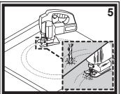
5) Drill a pilot hole on the inside edge of the inner line, larger enough for the jigsaw blade to fit in and cut the counter-top opening with the jigsaw. Choose the correct cutting tools for your counter-top material.
