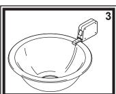
3) Measure the width of the flange of your particular sink model. Measure from the inside edge of the bowel to the outside edge of the flange.
