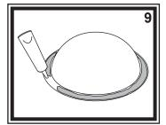
9) Apply a generous amount of marine grade adhesive sealant to the bottom of the flange. Consult your marine supplier for adhesive options.
