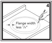
4) Draw a second line inside the outer traced line approximately 1/4" less then the flange's width to be used as the cut-out line. For example, if your flange is 1" wide, draw your second line 3/4" inside the traced outer line, if 1 1/4" flange = 1" inside, if 1 1/2" flange = 1 1/4" inside, if 1 3/4" flange = 1 1/2" inside = 1 1
