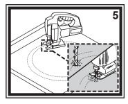
Drill a pilot hole on the inside edge of the inner line, larger enough for the jigsaw blade to fit in and 5) cut the counter-top opening with the jigsaw. Choose the correct cutting tools for your counter-top material.
