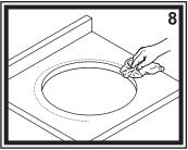
8) Clean the counter-top in preparation for the sink. Erase the pencil lines used for making the counter-top cutout and clean the surface of the counter. Counter-top will need to be clean and dry for sealant to adhere.
