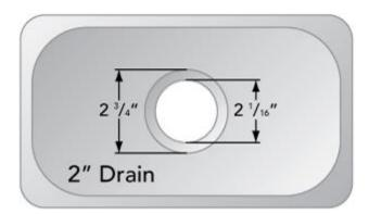
Sinks with 2" drains can be used as galley or head sinks. 2" drains are the standard size drain for most sinks Europe and the rest of the world. The name, 2" Drain, does not refer to the specific size of the hole in the sink or diameter of the drain, but is used as a standard term.
