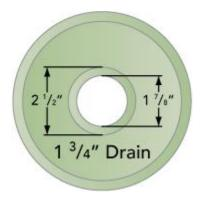
Glass vessel sinks use a 1 3/4" drain and are generally used as head sinks. 1 3/4" drains are the standard size drain for vessel sinks in North America and Europe. The name, 1 1/2" Drain, does not refer to the specific size of the hole in the sink or diameter of the drain, but is used as a standard term.
