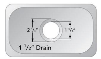
Sinks with 1 1/2" drains are generally used as head sinks. 1 1/2" drains are the standard size drain for lavatory sinks in North America. The name, 1 1/2" Drain, does not refer to the specific size of the hole in the sink or diameter of the drain, but is used as a standard term.
