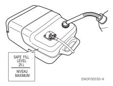
After filling the tank, close the fuel tank cap until two clicks sound is heard. ENOM00037-A
