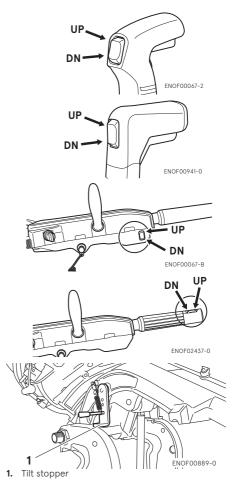
The outboard motor can also be tilted up and down using the switch provided under the bottom cowl.
