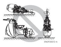
Keep the outboard motor in a vertical position when carrying.
