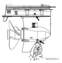
Install the upper oil plug, and then remove oil tube nozzle and install the lower oil plug. Oil plug specified tightening torque **4N·m (3 ft·lb, 0.4 kgf·m)**
