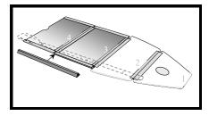
This lifts the floorboards up to have easier access to put the stringers on the sides of the floor.
