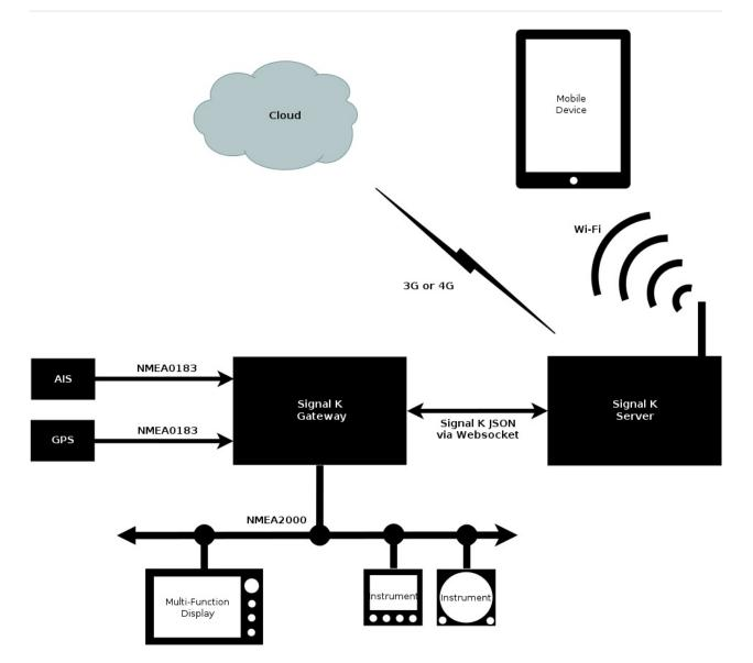
One major advantage of Signal K is the ability to represent data from heterogeneous sources. In addition to traditional NMEA sources data from generic sensors as well as modern Signal K enabled sensors can be fused into a single data model and a single protocol for accessing the data. Another typical setup is a Signal K server with adapters and converters for the different sources.
