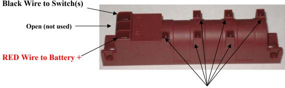
Spark Plug wires (not location specific) Unused terminals need to be grounded.
