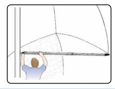
1 Un-Cleat The Line 2 Pull Line To Extend The Pole 3 Re-Cleat The Line.
