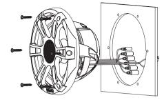
**16** Secure the speaker to the mounting surface using the included screws.
