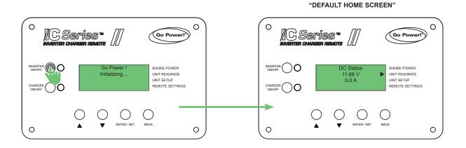
1. Press the Inverter ON/OFF button to turn the Inverter on, which then automatically powers the remote up. The remote will take up to 10 seconds to go to the default home screen which is DC Status in the unit readings sub menu. As shown above.
