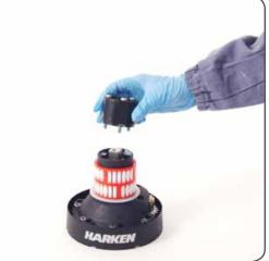
6. Completely unscrew the three screws n° 27 7. Remove the self-tailing arm support n°21
