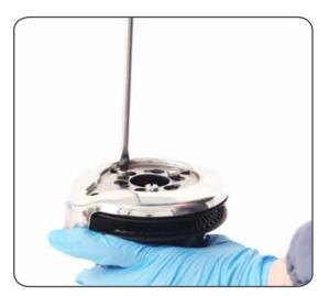
3. Unscrew the three screws n°27 ( $^{\circ}_{4}$ 4Nm/35 in-lb)
