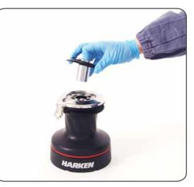
2. Slide off the hub  $n^\circ 28$  and the cover  $n^\circ 29$
