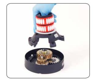
10. Remove the drum support n°15 Important: washer n°12 may remain inside the drum support!
