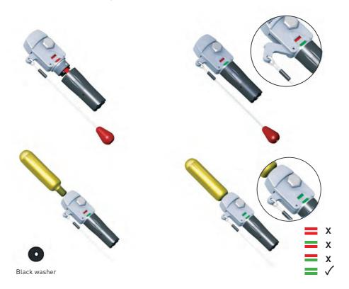
Un-screw anti-clockwise and remove gas cylinder. Whilst the gas cylinder is removed, examine the firing head and rubber gas seal make shore when testing that the manual inflation lanyard returns freely and that it is in the closed position. Test its operation by pressing on the cutter pin to see if it travels freely, the unit sensor will show green when testing.
