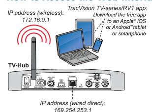
You can access the web interface using any Wi-Fi-enabled mobile device (such as a smartphone, tablet, or laptop).
