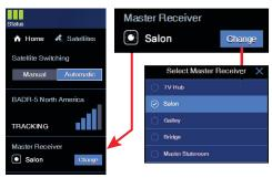
If your system is set up for automatic satellite switching with multiple receivers, you can select the master receiver on the Home page of the web interface. The master receiver controls satellite selection.
