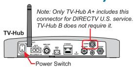
At the rear panel of the TV-Hub, set the power switch to the On position. The TV-Hub supplies power to the antenna. Wait a few minutes for system startup.
