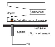
**Note:** If it is not possible to align the sensor and magnet exactly the AA grey sensor may be fitted up to 20mm out of alignment. The AA black sensor and the reed switch sensor must be directly aligned.
