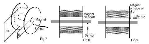
Gap Between the Sensor and Magnet:
