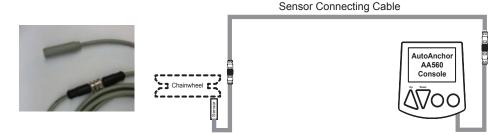
The sensor cable and the console sensor cable are fitted with female plugs. Sensor connecting cable with a male plug at each end is available in the following lengths:
