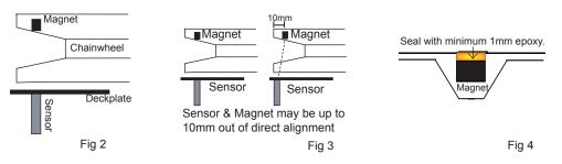
**Magnet Size:** 10mm X 8mm magnet (#9061). An 8mm x 6mm magnet (#9052) may be used on smaller windlasses. Check with your supplier.
