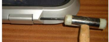
2. Use punch to push pin 2mm into hole
