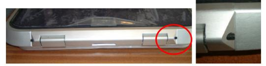
5. Clamp a pair of mole grips on to the part of the hinge pin which is sticking out. Withdraw the hinge pin
