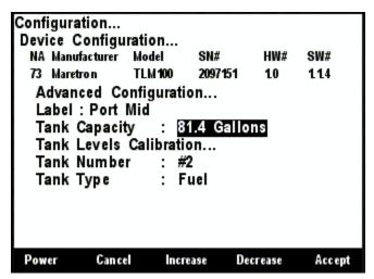
Figure 205 – Configuring the Tank Capacity
