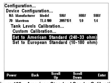
Figure 195 – American Standard Sender Calibration
