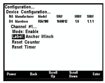
Figure 158 - RIM100 Channel Configuration Screen
