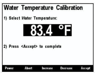
Figure 33 – Airmar Temperature Transducer Water Temperature Calibration Screen
