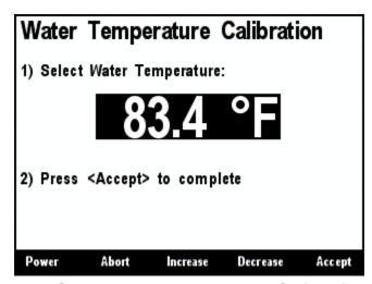
Figure 80 - DST110 Water Temperature Calibration Screen
