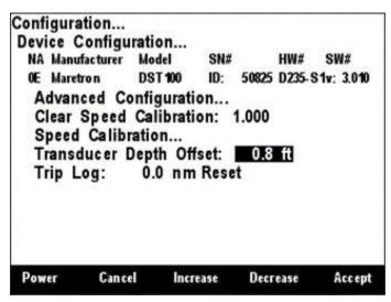
Figure 74 – Setting the Transducer Depth Offset in a DST100
