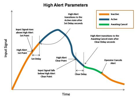
Figure 276 - High Alert Parameters
