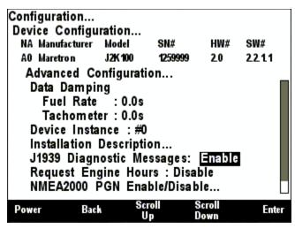
Figure 132 – J2K100 J1939 Diagnostic Messages Configuration
