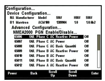
Figure 42 – ACM100 NMEA 2000® PGN Enable/Disable Screen
