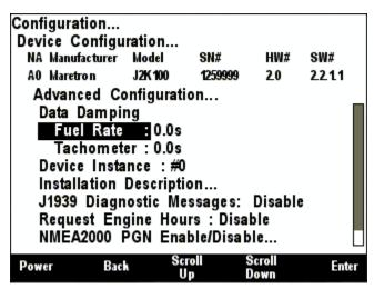
Figure 131 – J2K100 Advanced Configuration Screen
