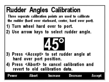
Figure 149 – RAA100 Port Rudder Angle Calibration
