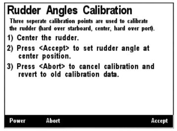
Figure 148 – RAA100 Center Rudder Angle Calibration
