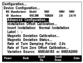
Figure 167 - SSC200/SSC300 Configuration Screen
