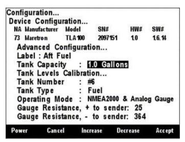
Figure 187 – Configuring the Tank Capacity
