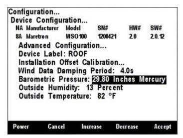
Figure 233 – Setting the Barometric Pressure
