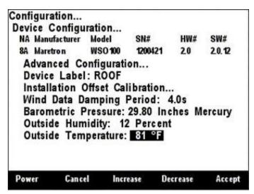
Figure 235 - Setting the Outside Temperature
