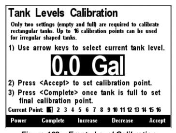
Figure 102 – Empty Level Calibration
