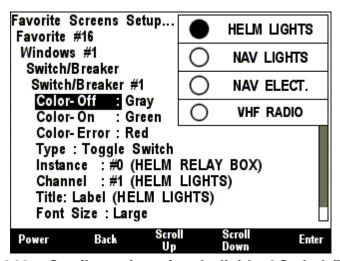
Figure 268 – Configuration of an Individual Switch/Breaker
