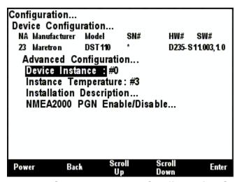
Figure 77 – DST110 Advanced Configuration Screen
