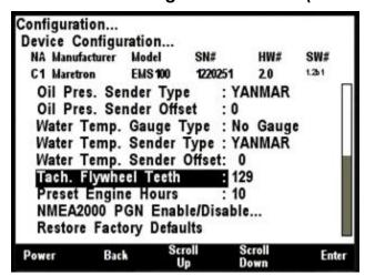
Figure 84 – EMS100 Configuration Screen (Second Screen)
