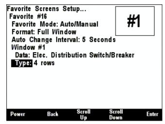
Figure 266 - Configuration of Switch/Breaker Display
