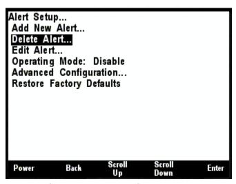
Figure 294 – Deleting an Alert
