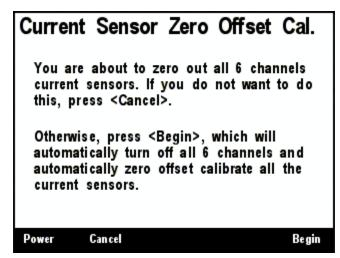
Figure 53 - DCR100 Current Sensor Zero Offset Calibration Screen
