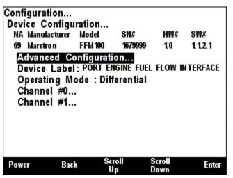
Figure 85 - FFM100 Configuration Screen
