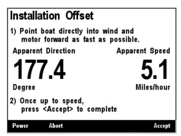
Figure 228 - WSO100 Installation Offset Screen
