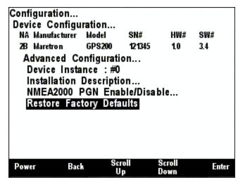
Figure 122 – Restoring Factory Defaults on the GPS200
