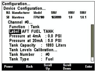
Figure 98 – FPM100 Channel #0 First Configuration Screen (Tank Mode)
