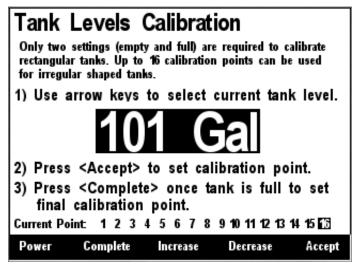
Figure 104 - Full Level Calibration
