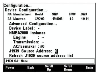
Figure 138 – J2K100 J1939 Source Address Configuration
