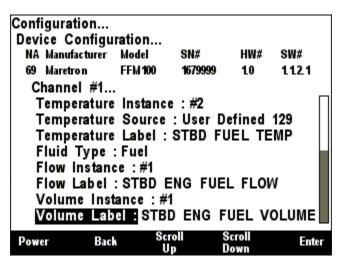
Figure 94 – FFM100 Channel #1 Second Configuration Screen (Two Independent Sensors Mode)
