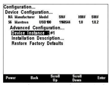
Figure 220 – USB100 Advanced Configuration Screen
