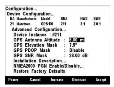
Figure 110 – Configuring Antenna Altitude on a GPS100
