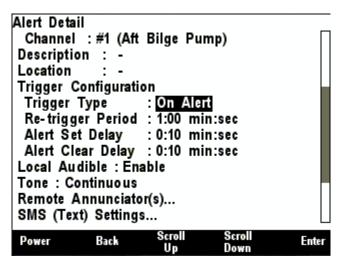
Figure 281 - Trigger Configuration - On Alert
