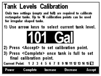
Figure 193 - Full Level Calibration
