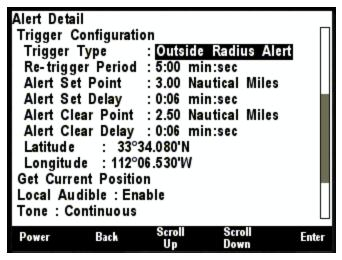
Figure 285 – Trigger Configuration – Outside Radius Alert
