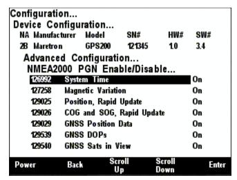
Figure 121 – GPS200 NMEA 2000® PGN Enable/Disable Screen
