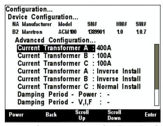
Figure 41 – ACM100 Advanced Configuration Screen
