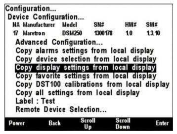
Figure 64 – DSM150/DSM250/DSM410/DSM570 Copy display settings from local display
