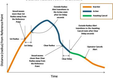
Figure 284 - Outside Alert Parameters
