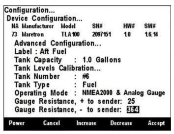
Figure 201 – Configuring the - to Sender Gauge Resistance
