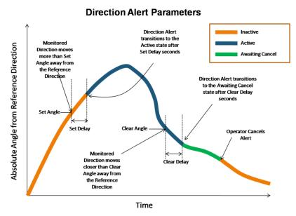
Figure 288 – Direction Alert Parameters
