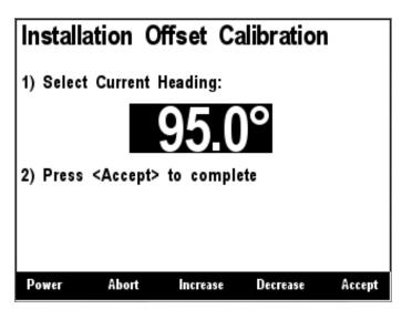
Figure 173 – SSC200/SSC300 Installation Offset Calibration Screen
