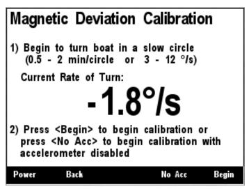
Figure 175 – SSC200/SSC300 Magnetic Deviation Calibration Start Screen
