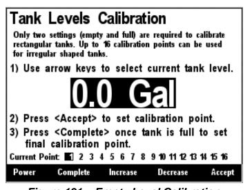
Figure 191 – Empty Level Calibration
