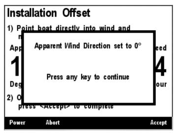
Figure 230 – Installation Offset Success Confirmation Screen
