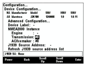
Figure 136 – J2K100 NMEA2000 Transmission Instance Configuration
