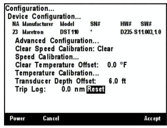
Figure 82 - Resetting the DST110 Trip Distance Log
