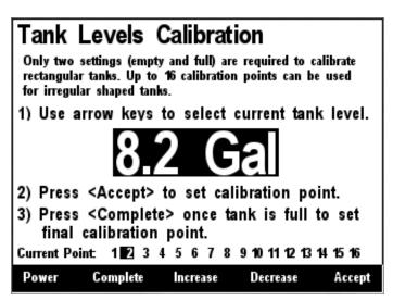
Figure 192 – Intermediate Level Calibration
