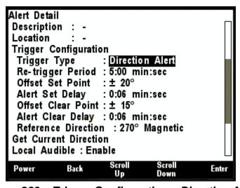
Figure 289 – Trigger Configuration – Direction Alert
