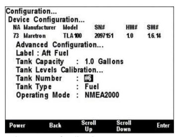
Figure 197 – Configuring the Tank Number
