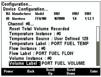
Figure 89 – FFM100 Channel #0 Second Configuration Screen (Differential Mode)
