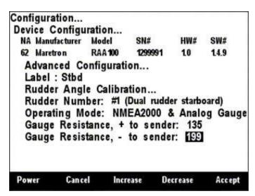
Figure 154 – RAA100: Setting the – to Sender Gauge Resistance
