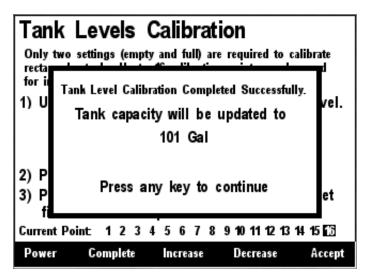
Figure 212 – Custom Tank Level Calibration Confirmation Screen
