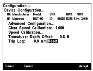
Figure 75 - Resetting the DST100 Trip Distance Log
