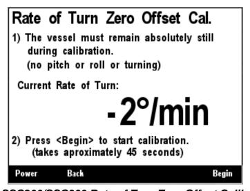
Figure 179 – SSC200/SSC300 Rate of Turn Zero Offset Calibration Screen
