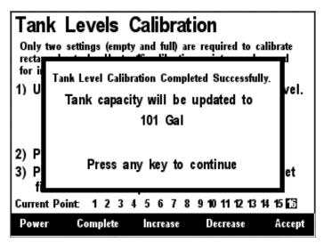
Figure 194 – Custom Tank Level Calibration Confirmation Screen
