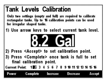
Figure 210 – Intermediate Level Calibration
