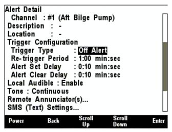
Figure 282 – Trigger Configuration – Off Alert
