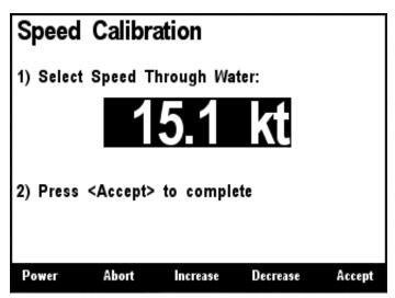
Figure 32 - Calibrating the Airmar Speed Transducer Speed
