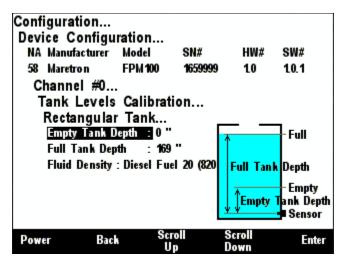
Figure 106 – Rectangular Tank Calibration
