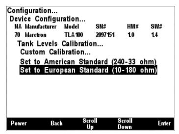
Figure 196 – European Standard Sender Calibration
