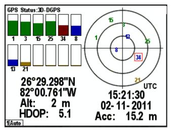
Figure 244 - GPS Status Display Example
