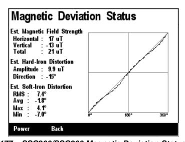
Figure 177 – SSC200/SSC300 Magnetic Deviation Status Screen
