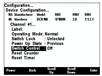
Figure 56 – DCR100 Channel Configuration Screen (DCR Mode)
