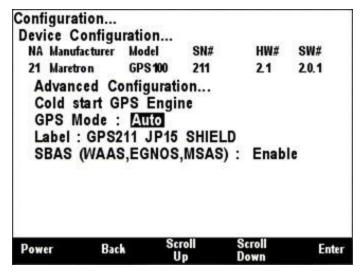
Figure 117 – Configuring GPS Operating Mode on a GPS100
