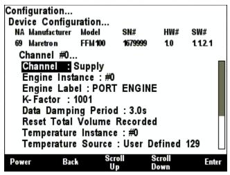
Figure 88 – FFM100 Channel #0 First Configuration Screen (Differential Mode)
