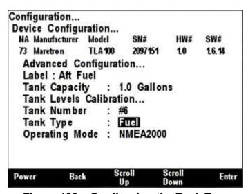
Figure 198 – Configuring the Tank Type
