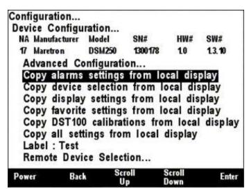
Figure 62 – DSM150/DSM250/DSM410/DSM570 Copy alarms settings from local display
