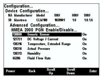
Figure 49 - CLM100 NMEA 2000® PGN Enable/Disable Screen
