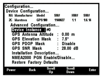
Figure 109 – GPS100 Advanced Configuration Screen
