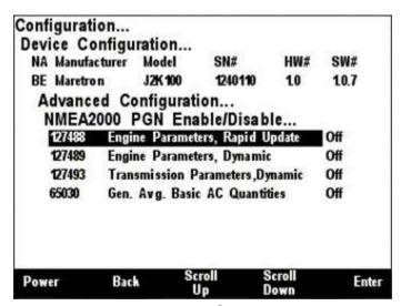
Figure 134 – J2K100 NMEA 2000® PGN Enable/Disable Screen
