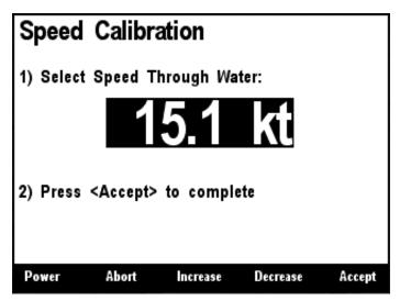
Figure 79 – Calibrating the DST110 Speed
