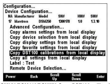
Figure 67 – DSM150/DSM250/DSM410/DSM570 Copy DST100 calibrations from local display
