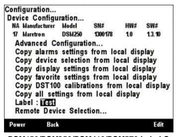
Figure 69 – DSM150/DSM250/DSM410/DSM570 Label Configuration
