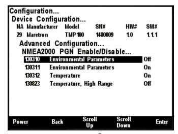
Figure 217 – TMP100 NMEA 2000® PGN Enable/Disable Screen
