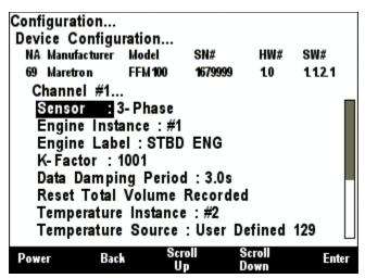
Figure 93 – FFM100 Channel #1 First Configuration Screen (Two Independent Sensors Mode)
