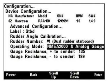
Figure 152 – RAA100: Setting the Operating Mode
