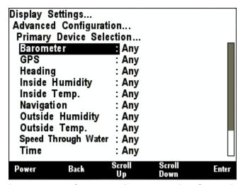
Figure 12 – DSM570 Primary Device Selection
