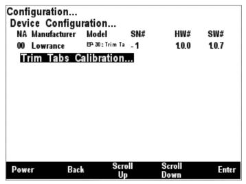
Figure 36 – EP-30 Trim Tabs Configuration Screen
