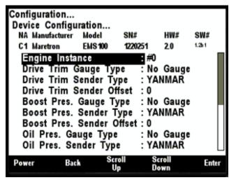
Figure 83 - EMS100 Configuration Screen (First Screen)
