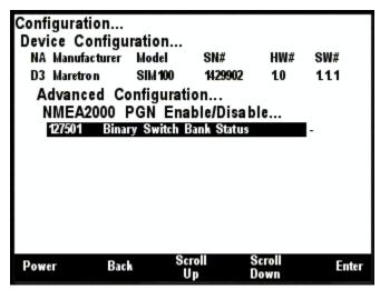
Figure 161 - SIM100 NMEA 2000® PGN Enable/Disable Screen
