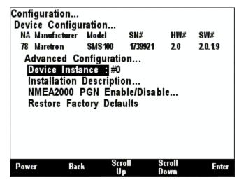
Figure 164 – SMS100 Advanced Configuration Menu
