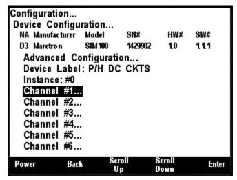
Figure 159 – SIM100 Configuration Screen
