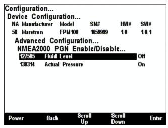
Figure 97 – FPM100 NMEA 2000® PGN Enable/Disable Screen
