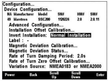
Figure 174 – Setting the Installation Orientation
