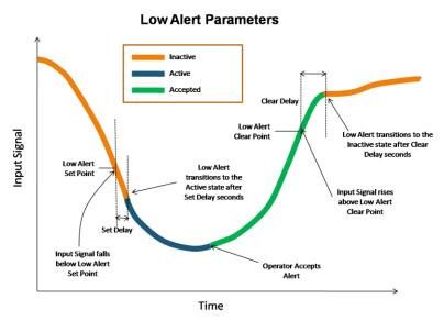
Figure 278 - Low Alert Parameters
