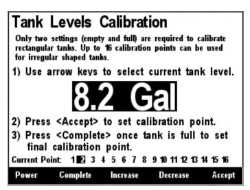
Figure 103 – Intermediate Level Calibration
