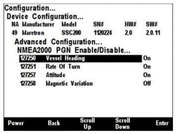
Figure 172 – SSC200/SSC300 NMEA 2000® PGN Enable/Disable Screen
