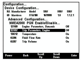
Figure 87 - FFM100 NMEA PGN Enable/Disable Screen
