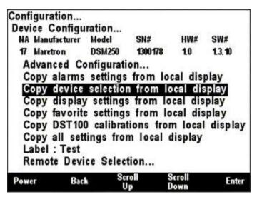
Figure 63 – DSM150/DSM250/DSM410/DSM570 Copy device selection from local display
