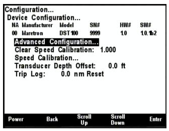
Figure 71 – DST100 Configuration Screen
