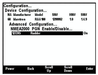
Figure 143 – RAA100 NMEA 2000® PGN Enable/Disable Screen
