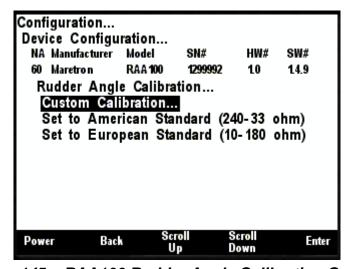
Figure 145 – RAA100 Rudder Angle Calibration Options
