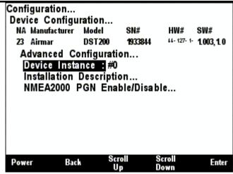
Figure 31 - Airmar Transducer Advanced Configuration Screen
