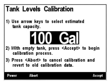
Figure 190 – Tank Levels Calibration Capacity Estimation
