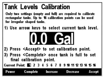
Figure 209 - Empty Level Calibration
