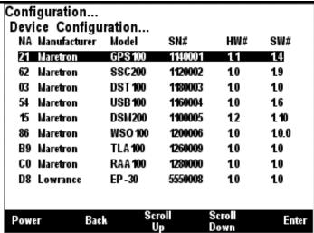
Figure 29 - Device Configuration Screen
