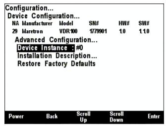
Figure 223 - VDR100 Advanced Configuration Screen
