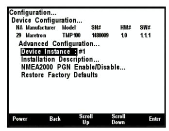
Figure 216 – TMP100 Advanced Configuration Screen
