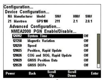
Figure 114 – GPS100 NMEA 2000® PGN Enable/Disable Screen
