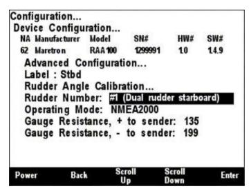
Figure 151 – RAA100: Setting the Rudder Number
