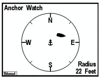
Figure 236 - Anchor Watch Display Example
