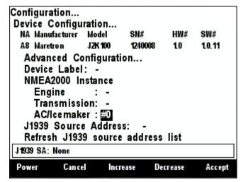
Figure 137 – J2K100 NMEA2000 AC/Icemaker Instance Configuration
