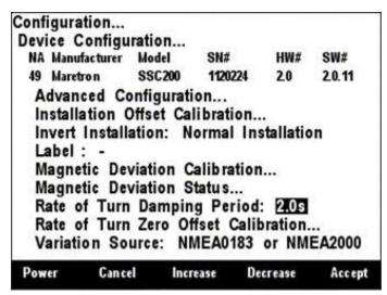
Figure 178 - Programming SSC200/SSC300 Rate of Turn Damping Period
