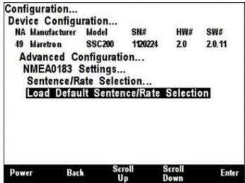
Figure 171 – SSC200/SSC300 Load Default Periodic Rate Selection
