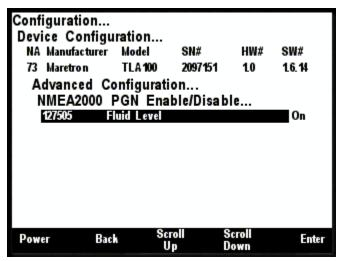
Figure 186 - TLA100 NMEA 2000® PGN Enable/Disable Screen
