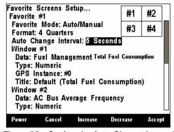
Figure 25 – Setting the Auto Change Interval
