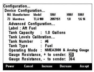
Figure 200 – Configuring the + to Sender Gauge Resistance
