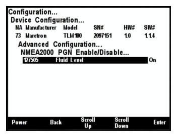
Figure 204 – TLM100 NMEA 2000® PGN Enable/Disable Screen
