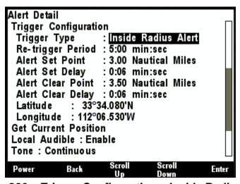
Figure 286 - Trigger Configuration - Inside Radius Alert
