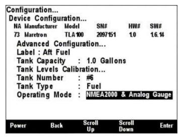
Figure 199 – Configuring the Operating Mode
