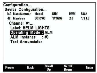
Figure 57 – DCR100 Channel Configuration Screen (ALM Mode)
