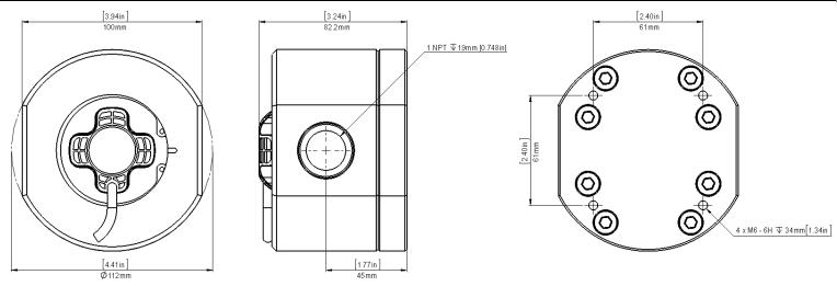
Figure 3 - Fuel Flow Sensor Mechanical Drawing
