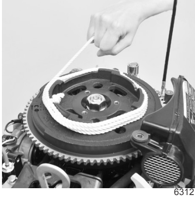
Emergency start rope on flywheel
