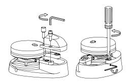
6. Re-fit the chain cover and tighten the thumb or socket head cap screw as appropriate.
