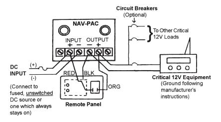
3) Remote Panel: Mount in a conspicuous location where the loss of power indication will be noticed. The NAV-PAC will function normally without the remote panel or with the remote panel switch off. Connect the wiring as follows: (see diagram)
