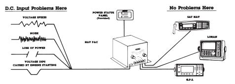
The NAV-PAC protects electronics from voltage spikes, power surges, momentary power losses, abrupt voltage changes and noise interference on incoming DC power to LORAN, SAT-NAV, GPS, CHART PLOTTERS and other Navigation Electronics prone to memory loss or "crashes".
