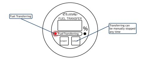
If the ship's power is removed during fuel transfer the transfer will stop. For safety reasons when the power is restored the unit will NOT restart the transfer unless the START button is depressed again or the automatic start feature is enabled and the tank level is below the user settable threshold.
