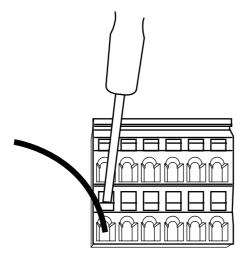
The cables from the power-source to the external sockets are connected using the WAGO Cage Clamp terminal block. The wire should be stripped for 8mm and then the cage clamp opened with a small screwdriver in the slot above the wire connection. Then simply insert the wire into it's connection slot and release the cage clamp by removing the small screw driver. This will produce a secure gas tight connection on wire sizes from 0.08 - 1.5 mm<sup>2</sup>
