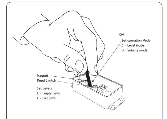
The 4-20mA Tank Level Adaptor can be calibrated to operate between the set Empty & Full level.
