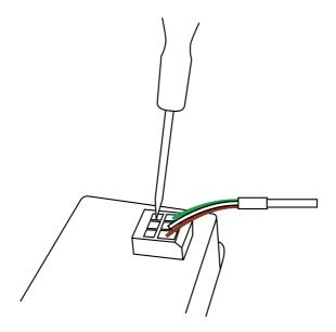
The wires from the Thermocouple Cable are connected to the WAGO cage clamp terminal block by placing a small screw driver in the slot above the terminal turning it to open the cage clamp. Insert the wire into the terminal block and withdraw the screwdriver to allow the cage clamp to make a good connection onto the bared wire end.
