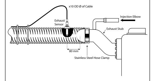
Use cable ties to prevent the stainless steel shrouded cable from chafe or damage.
