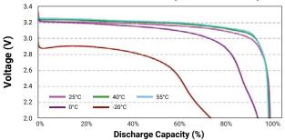
Charge: CC-CV 1C (max) 3.65V, 1250mA, cutt-off at 25°C Discharge: CC 1C, 2 0V cutt-off at different temperature
