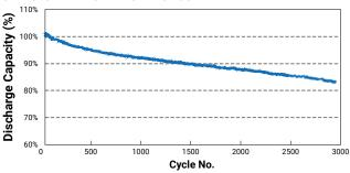
Charge: CC-CV 1C (max) 3.65V, 1250mA, cutt-off at 25°C Discharge: CC 1C, 2.0V cutt-off at 25°C
