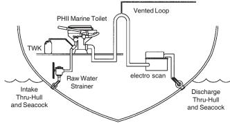
Electro Scan with Vented Loop (Above Waterline)
