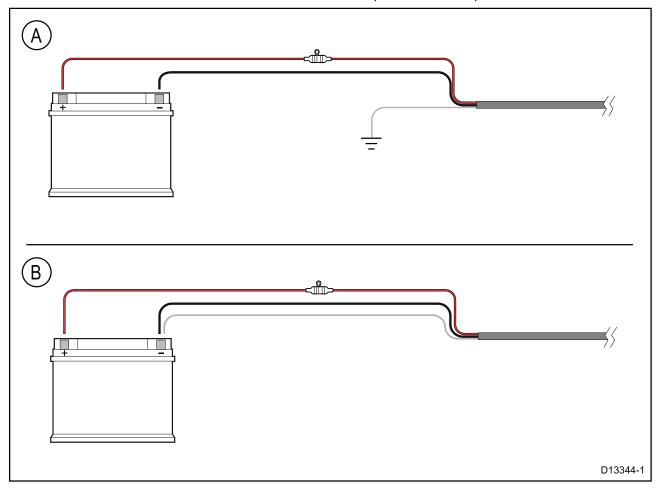
A Battery connection scenario A: suitable for a vessel with a common RF ground point. In this scenario, if your product's power cable is supplied with a separate drain wire then it should be connected to the vessel's common ground point.
