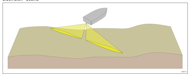
**SideVision**™ is effective at lower vessel speeds. The wide, thin beams produce clear target returns. As your vessel moves forward, subsequent returns build up to provide an image of the sea floor on each side of your vessel.
