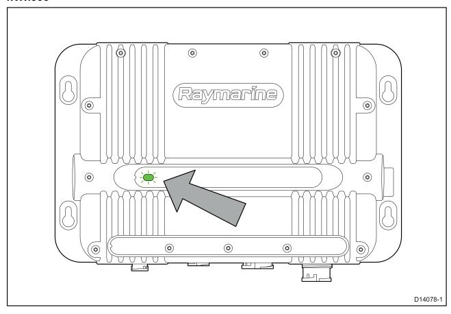
The LED on the front panel of the unit provides information on the status of the sonar module and notifies users of any problems within the unit. The LED blinks the following colors:
