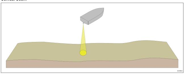
Sonar is effective at a range of speeds. In deeper waters the CHIRP bandwidth is automatically optimized to improve bottom lock and the detection of moving objects (e.g. fish) in the wider water column.
