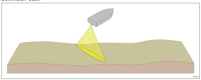
**DownVision**<sup>™</sup> is effective at lower vessel speeds. In deeper waters the CHIRP bandwidth is automatically optimized to improve bottom lock and the detection of moving objects (e.g. fish) in the wider water column.
