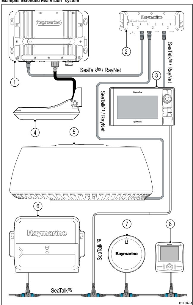
**Note:** Power connections are not shown in this illustration. The sonar module, multifunction display, and some of the other devices shown require their own dedicated power connection.
