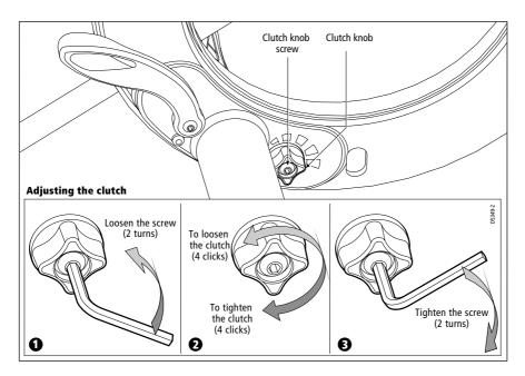
You need to adjust the clutch if you have removed the clutch eccentrics, replaced the ratchet knob, or replaced the drive belt. When the clutch is correctly adjusted:
