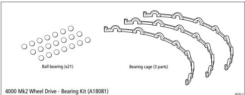
To replace the drive ring and/or ball bearings and/or bearing cage:
