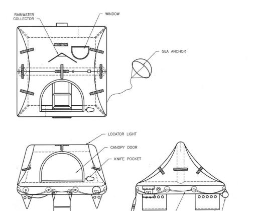
FIGURE 1A REVERE COASTAL ELITE LIFERAFT SHOWN INFLATED
