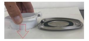
6. When cup has been pushed back, flush with mounting surface, replace the mounting screws. Be careful to not overtighten the screws, as this may crack the mounting cup.
