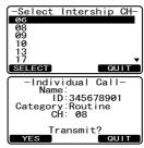
12. Press the QUIT soft key to listen to the channel to make sure it is not busy, then press the microphone's **PTT** switch and talk into the microphone to the other vessel.
