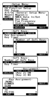
Press the QUIT key, then rotate the CH knob to select "KEY TIMER" (selects how long the soft key icon will be shown on the display after a soft key is pressed, default is 5 seconds). Then, press the SELECT soft key.
