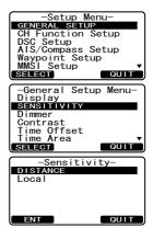
To return to normal sensitivity, repeat the above procedure, rotating the **CH** knob to select "DISTANCE" in step 5 above.
