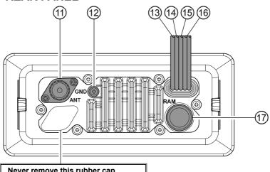
Never remove this rubber cap. When this rubber cap is removed, the water resistance performance is lost.
