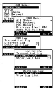
2) If you want to delete one of the logged stations, select the "VIEW LOG LIST" with the CH knob, then press the SELECT soft key. Rotate the CH knob to select the station (name or MMSI number) to be deleted, then press the DELETE soft key.
