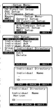
If a mistake was made entering in the name repeat pressing the SACK soft key until the wrong character is selected, then rotate the **CH** knob to correct the entry.
