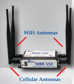
\*Wave WiFi's MBR550 Has a SIM slot for 3G/4G SIM cards.
