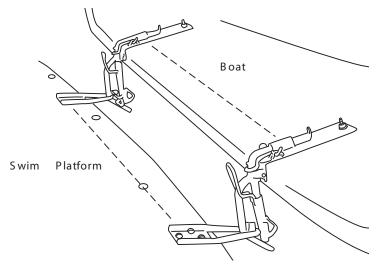
Step 2 - Mount both snap davits on dinghy over seating area or reinforced side using 1" bolts.
